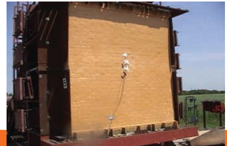
This 3-wythe brick masonry wall was retrofitted with 1/2" of Tyfo Blast-Flex. The average peak pressure was 10.65 psi with a maximum midspan deflection of 2.5".
