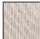
Tyfo® BC System Bi-directional glass composite (±45°)
