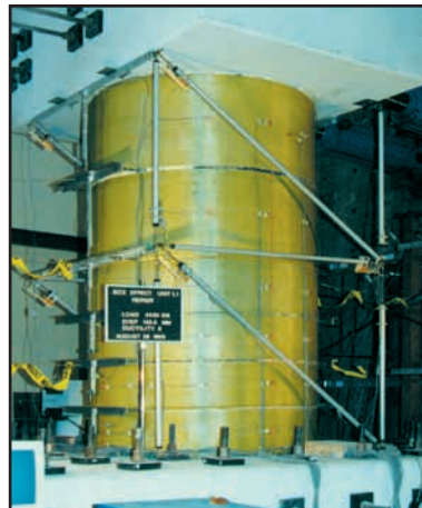
UCSD Column test with hysteresis loops
